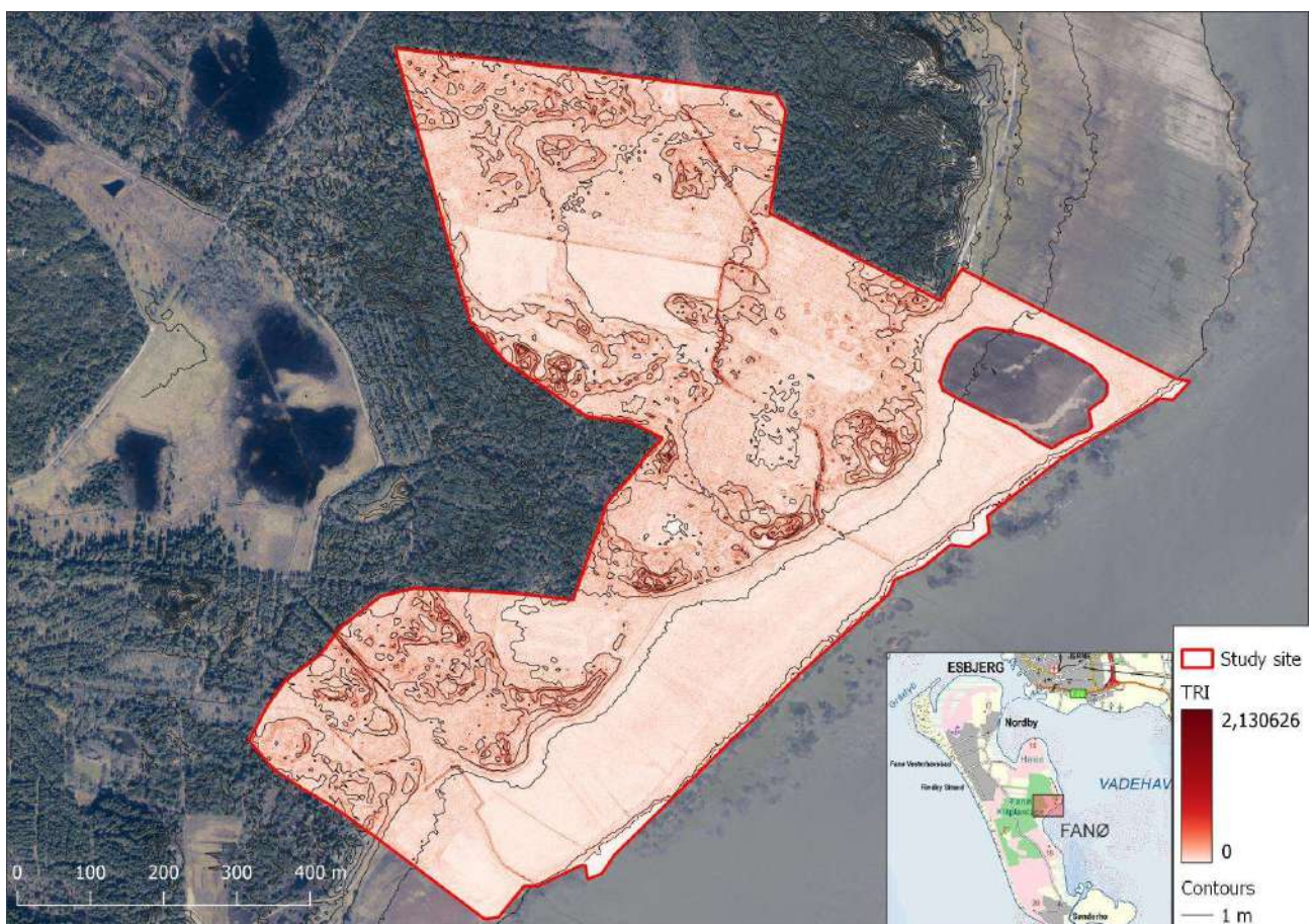
Figure 10: The figure shows the topography of the study site by terrain ruggedness analysis (TRI) and contours. The red colouration shows the TRI, where red colors indicate an increased variation of topography. The contours are shown with a 1-meter contour line.
